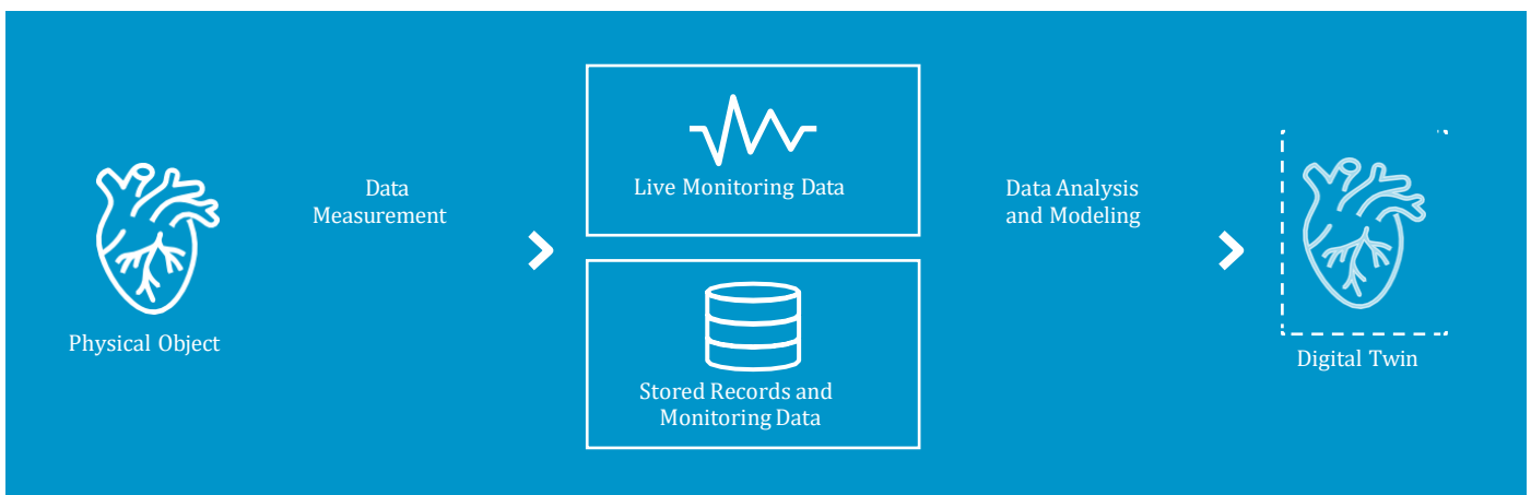
Figure 3. Digital twin of physical object, powered by live and historical data.
