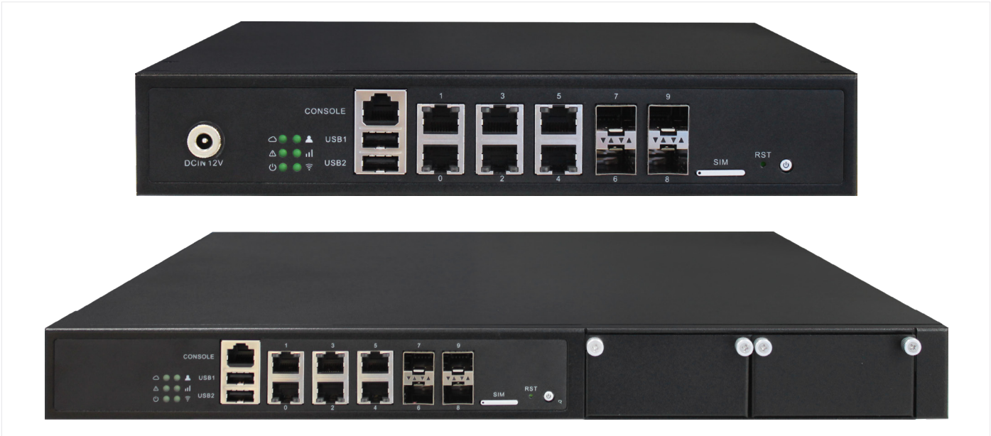
Figure 1. Two models of the uCPE 2.0 white box product; bottom version has two expansion bays.
