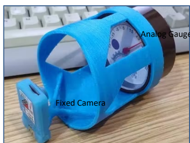
Figure 14 Image acquisition using a fixed camera
