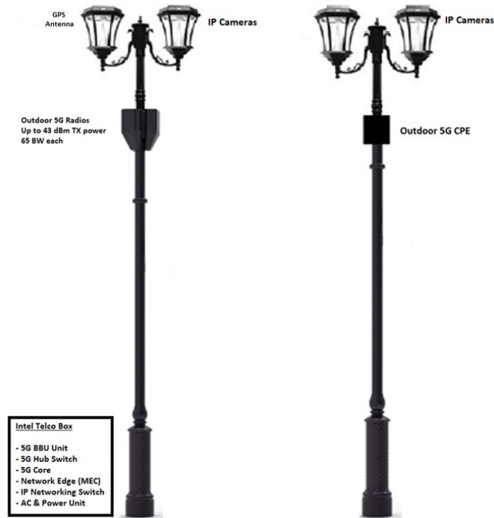
Figure 1 Intel Smart City Kit on City Light Poles
