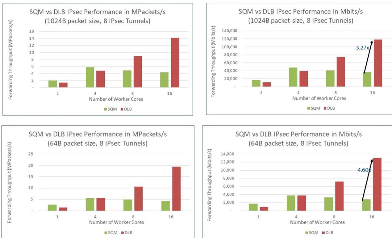
Figure 5. MPackets/s, Mbits/s Packet Performance Results (Top to Bottom) 1024B, 1 Tunnel; 64B, 1 Tunnel; 1024B, 8 Tunnels; 64B, 8 Tunnels
