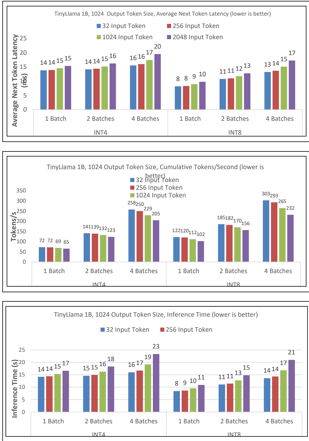
Figure 8. Generative AI Entry Configuration Performance Graph (TinyLlama with Intel® ARC380)
